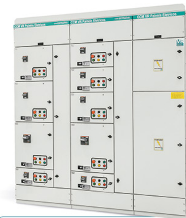
CCM- BT - Withdrawable Units - Form 4B TTA 65KA - Coord. Type 2
